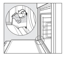
Prepare the door for removal. Flip up the locking clamps on each door hinge.
